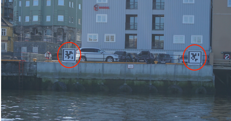
Figure 6.2: The AprilTag (Tag36h11 family) markers used in this thesis. The AprilTag marker on the right had id 0 and the marker on the left had id 1.
