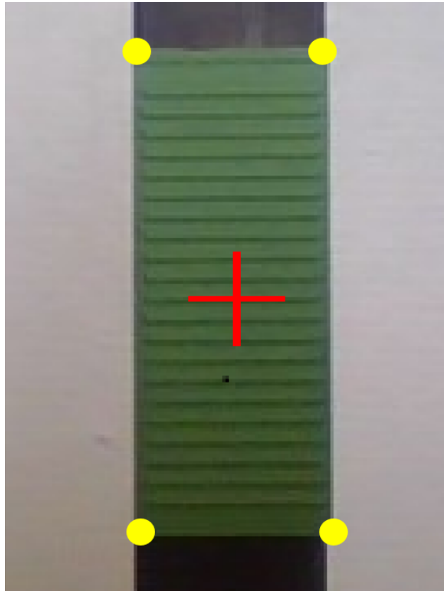
Figure 54: an array is created from these points, with an order starting from top left and moving horizontally towards the right. Similar to a rolling shutter movement. The origin of object frame is marked with a red cross
