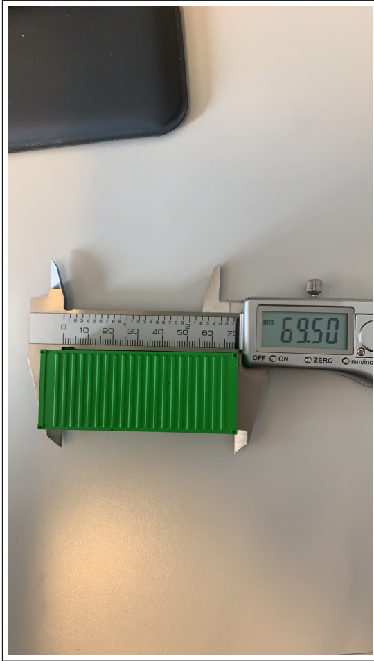
Figure 52: Length of container measured to be 69.50 mm
