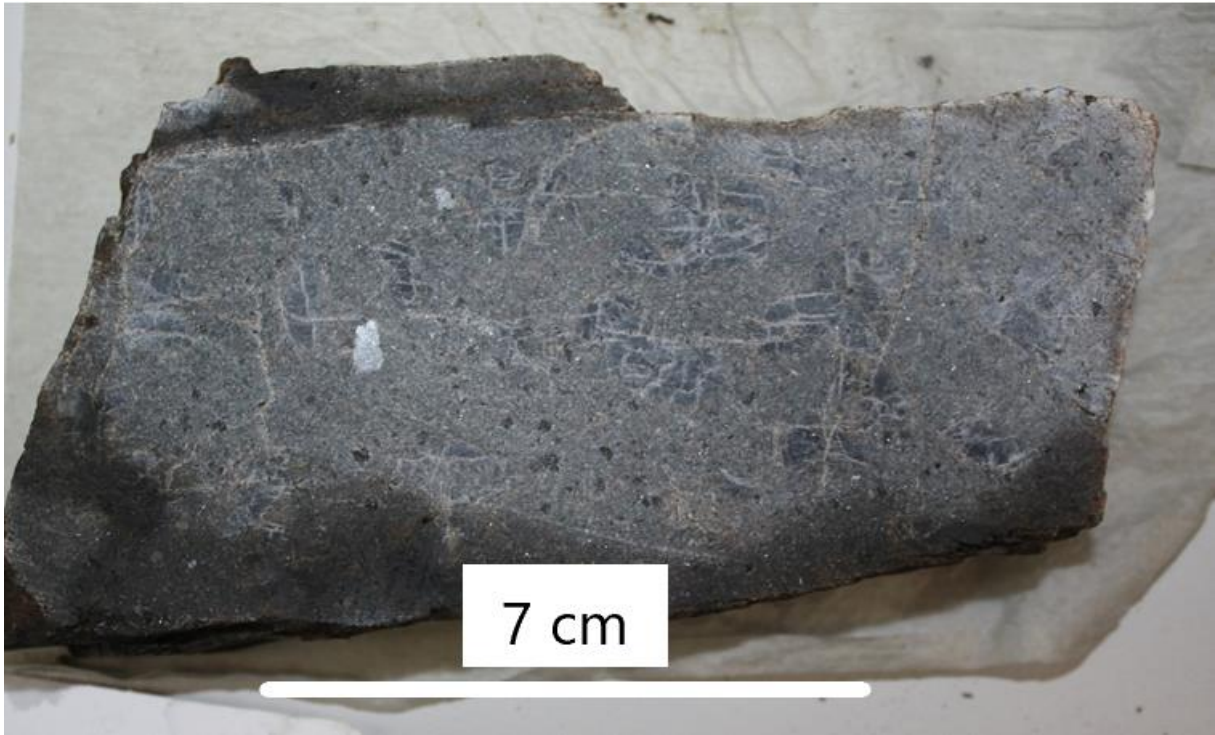
Figure 4-29: Slab photo of trachytic to porphyritic monzonite (512 B).
