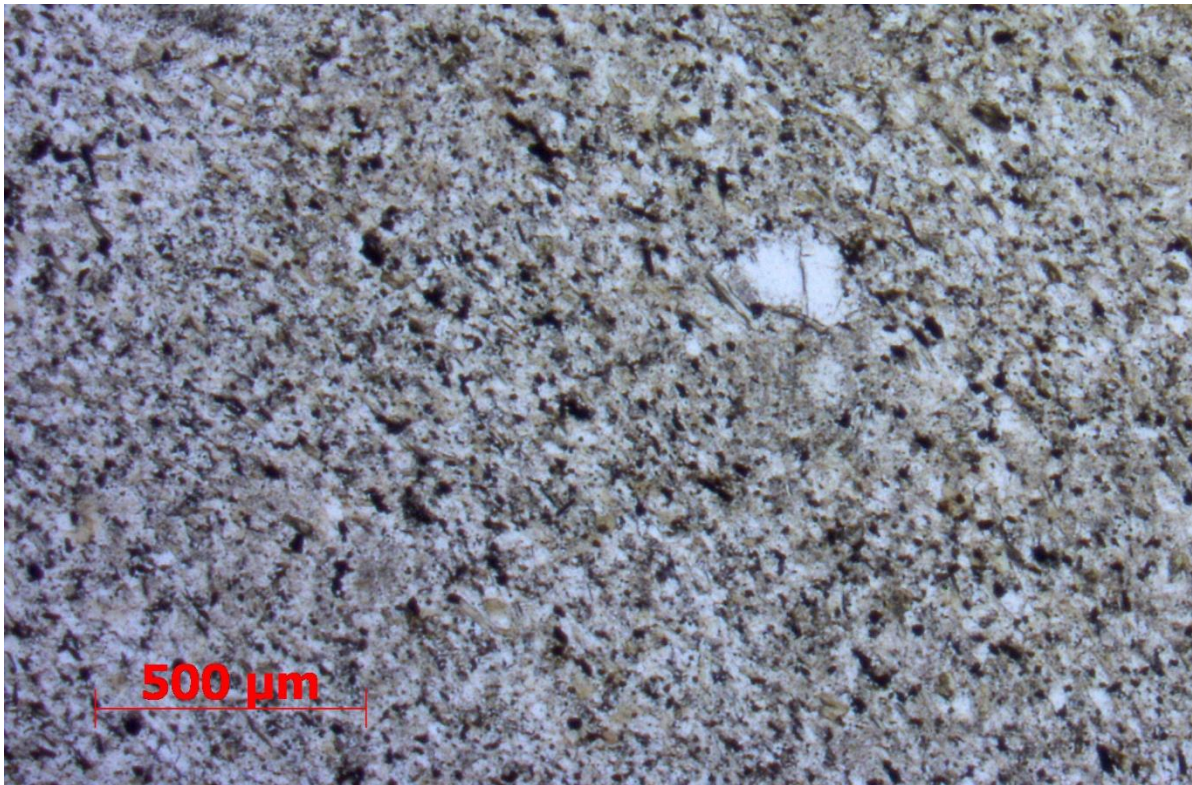
Figure 5-13: Photomicrograph of rhomb porphyry ground mass (524). Note elongated felspar (transparent) and Fe-Ti-oxides (opaque) show moderate orientation.
