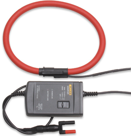
Figure 3.7: The Fluke i2000 flex used in laboratory testing [73].
