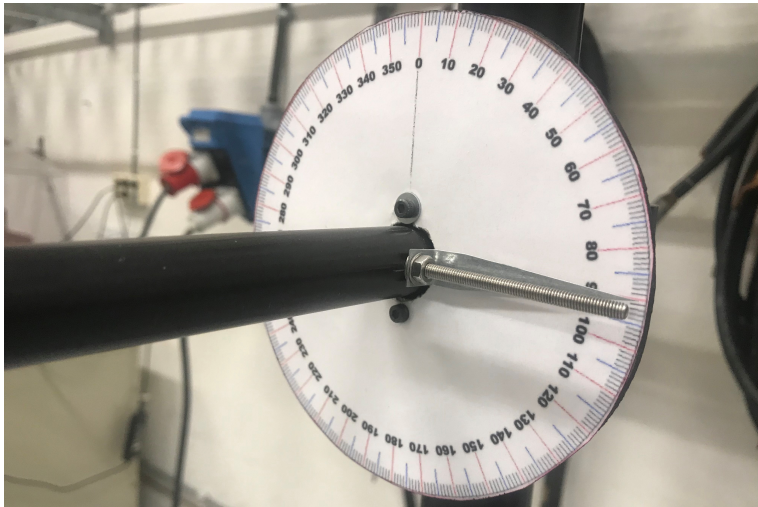
Figure A.7: Protractors for adjustment of conductor angle. Arrow indicator indicates the angle.
