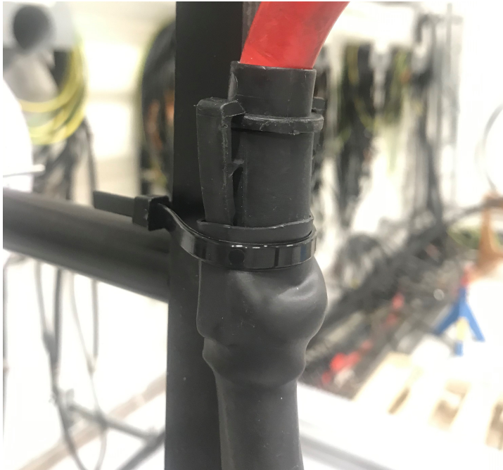
Figure A.5: Closeup of the RC discontinuity. The locking mechanism is located just above the strip.
