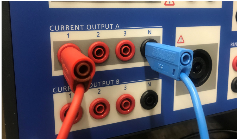
Figure A.3: Connection of the terminals to the Omicron current output using banana plugs. The current is outputted through current output A terminal one and returned on the neutral terminal. The schematic in figure A.1 uses the same color scheme, but the external conductor (bottom) is not connected.
