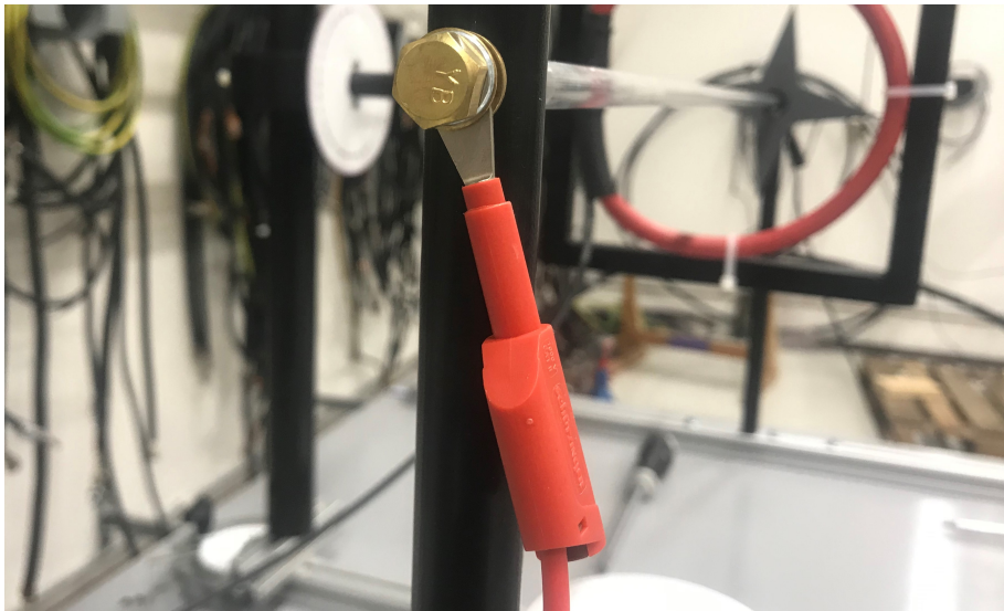
Figure A.4: The banana plug connected to the aluminium conductor with the RC in the background.
