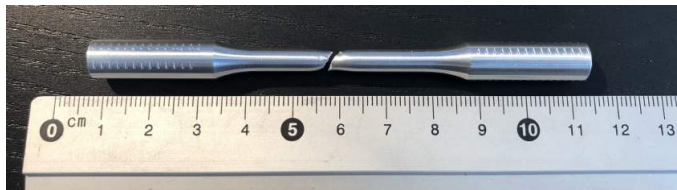
Figure G.2: MCSE 6060C T6b, fracture occurrence.
