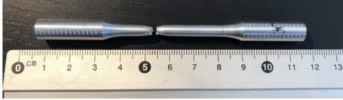
Figure G.5: RAM 6082 as-extruded, fracture occurrence.
