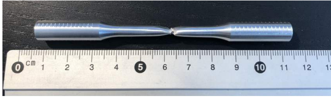
Figure G.6: RAM 6082 T6b, fracture occurrence.
