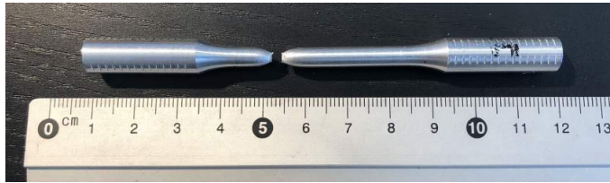
Figure G.1: MCSE 6060C as-extruded, fracture occurrence.
