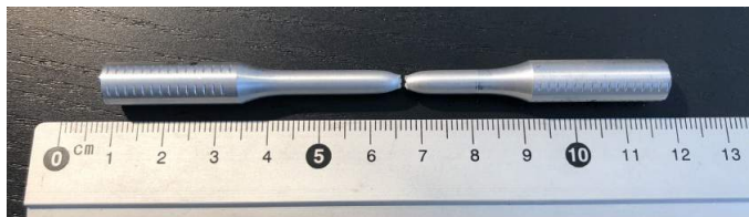
Figure G.3: MCSE 6082C as-extruded, fracture occurrence.
