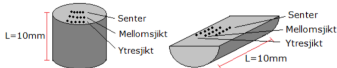
Figure 3.12: Hardness measurement indents on extruded profiles. From [62].
