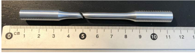
Figure G.4: MCSE 6082C T6b, fracture occurrence.
