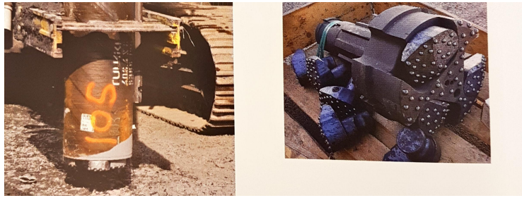
Figure 3.3.1: Shows the connection between the permanent "ring-bit" and the releasable "pilot-bit", taken from Statens vegvesen.
