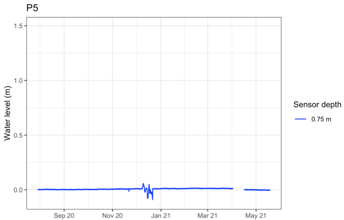
Figure 0.2 Water level within swale in sensor position P5 measured with pressure sensors.
