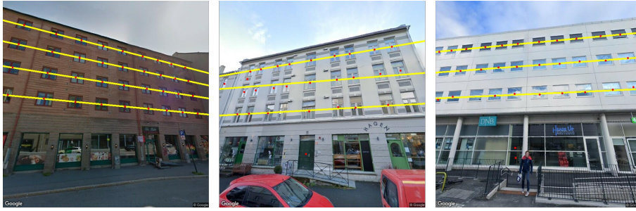
Figure 18: Visualization examples of the floor segmentation results on street-level imagery with undetected shop floors.
