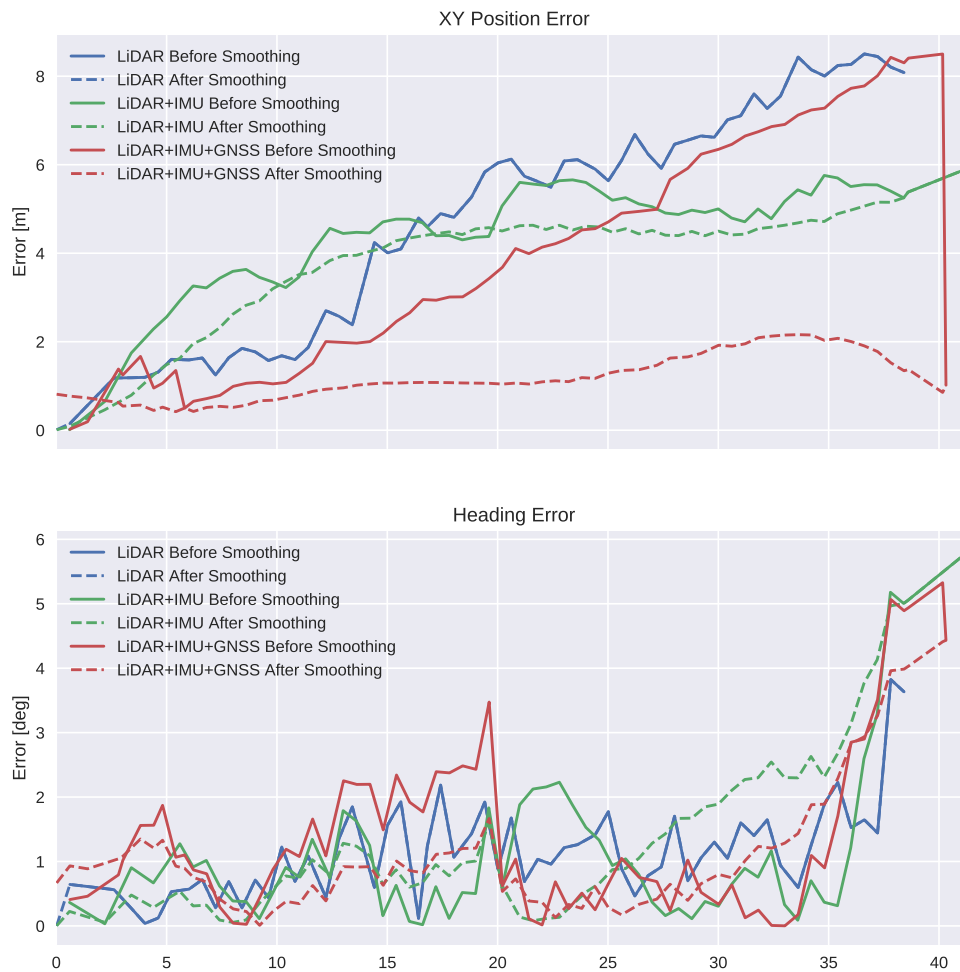
Figure 6.1: Sensor Comparison Experiment: The plot shows the absolute errors from the sensor comparisons experiments. Each experiment is plotted with the results before and after smoothing in the same color. The results before smoothing are plotted as a solid line, while the results after smoothing are plotted as a dashed line.
