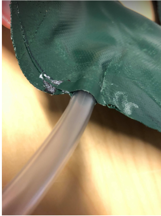
Figure 5.13: The tube used to inflate the inflatable element.
