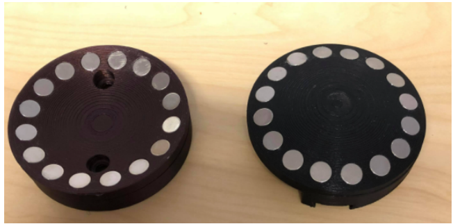
Figure 5.15: The sides of the magnetic connection with magnets.
