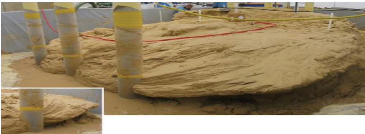
Figur 104. Show the exposed cemented sand body. Image from (Paassen, 2009)
