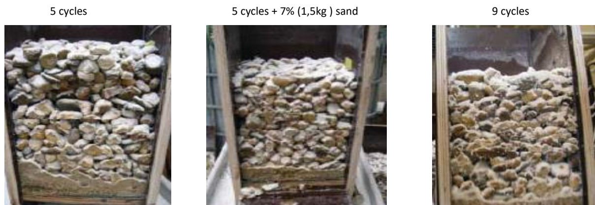
Figur 99. Show cementation for varying treatment strategies in coarse gravel. Images from (Van der Star et al., 2011)
