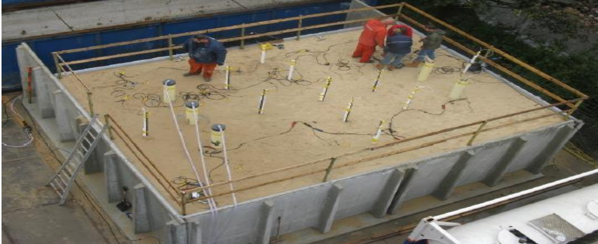
Figur 103. Show setup for larger scale MICP experiment in sand. Image from (Paassen, 2009)
