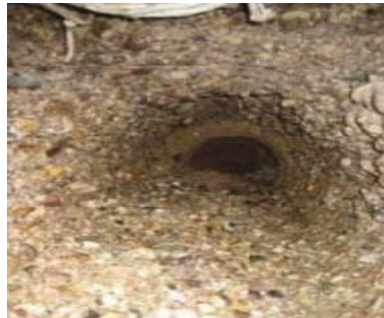
Figur 100. Shows drilling through cemented mass (left) and drilled pathway (right). Images from (Van der Star et al., 2011)
