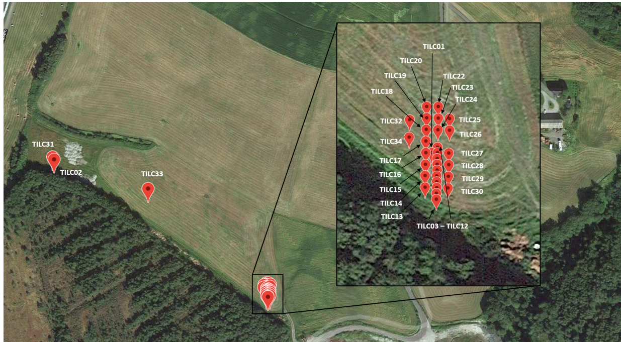
Figure 3.2: Location of the CPTu-soundings at Tiller-Flotten NGTS test site. Figure extracted from the NGTS quick-clay project, http://www.geocalcs.com/datamap .
