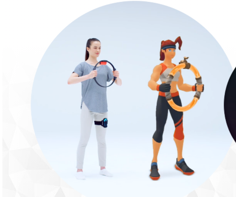
Figure 13.6: With one Joy-Con in the ring and one strapped to the leg the avatar can mimick the player's movements
