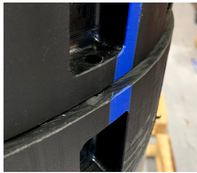
Figure 5.19: Deformation of pipe edges, resulting in big gaps between bolt holes.
