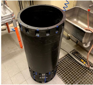
Figure 6.1: Joint 3 under waterproof test.
