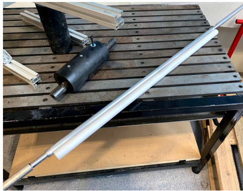
Figure 5.10: PP pipe and inner aluminum shaft of mandrel.
