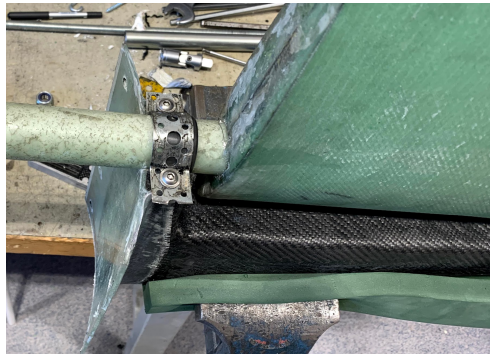
Figure 5.22: The rudder fastened to the skeg using a galvanized steel strip brace.
