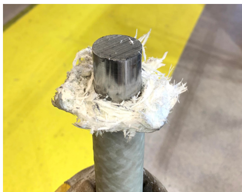
Figure 5.9: Delamination from excessive force during attempted demoulding.
