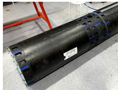
Figure 3.1: The extruded HDPE pipe used for the ORCA project
