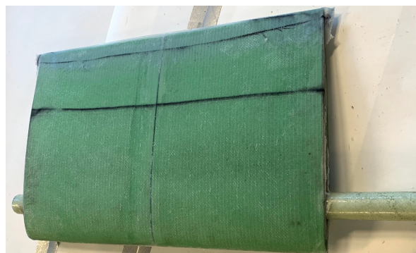
Figure 5.7: Overview of mouldless VARTM mid transfusion.
