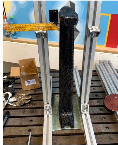
Figure 5.16: Rig made to measure skeg misalignment.
