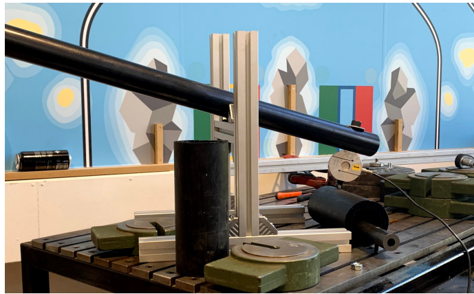
Figure 4.3: Experimental rig. With moment arm and load cell connected to the PE pipe.
