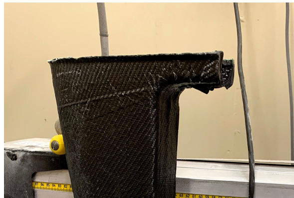
Figure 5.12: Wrinkles and surface imperfections in skeg.
