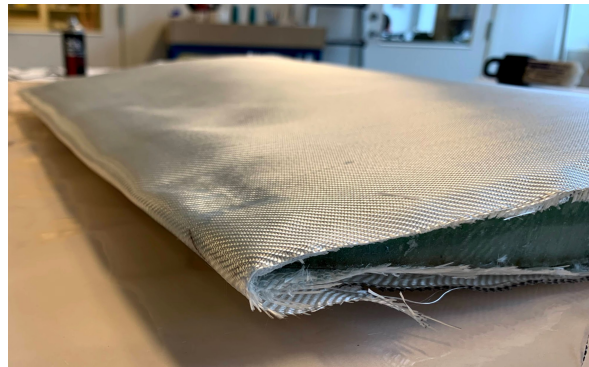
Figure 5.5: A close up of the cloth overlap at the trailing edge of the rudder.
