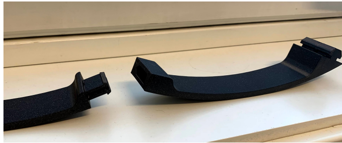
Figure 5.17: 3D printed profile support with snap connection.
