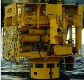
Figure 8: VXT made by FMC being lowered subsea [70]
