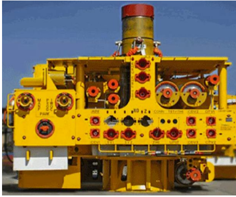
Figure 10: HXT made by FMC [70]
