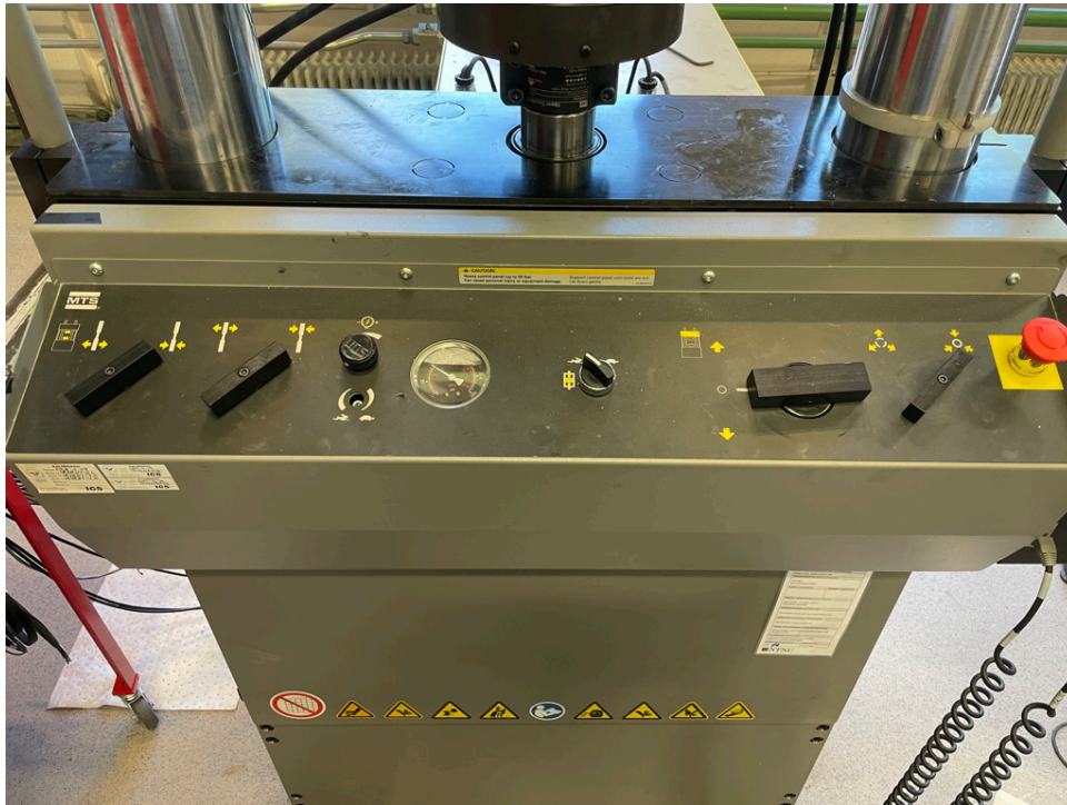
Figure 52: Control panel controlling gripping force. Has to be tuned to not be damaged while gripping
