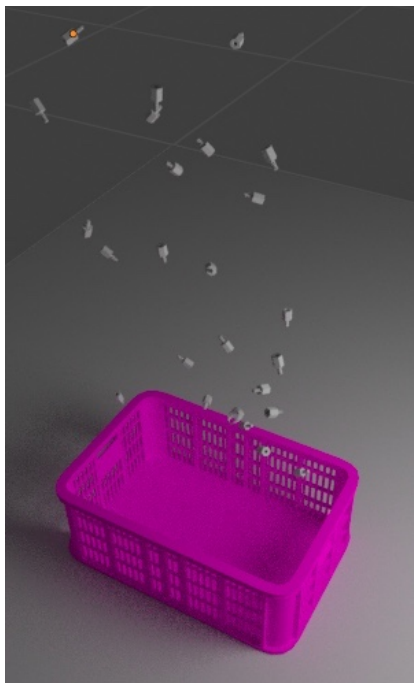
Figure 4.13.: Initial object poses generated by the ObjectManager class.
