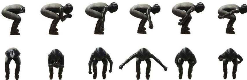
Figure 1: The model without arms and head, and different arm positions tested in this study. From the left: Without arms and head, baseline position, arms down, arms out, hands behind ankles and hands behind torso.
