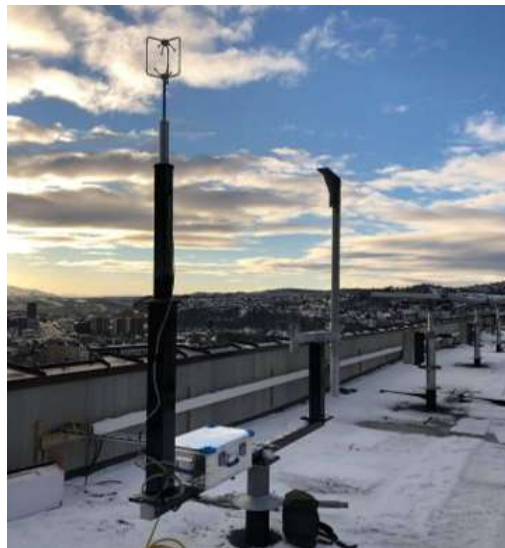
Figure 3.7: Anemometer mounted on the roof
