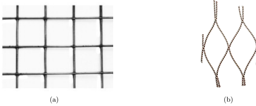
Figure 5: Physical net models used for the investigation of a copper net Welded-25 Tsukrov et al. (2011) and the twisted fabric net Zhou et al. (2015) in static current.
