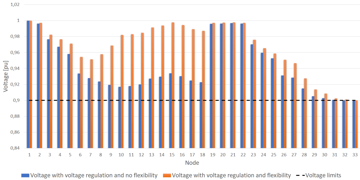
Figure 24: Voltage magnitude for all nodes with voltage regulation on node 33 for time period 08:15.
