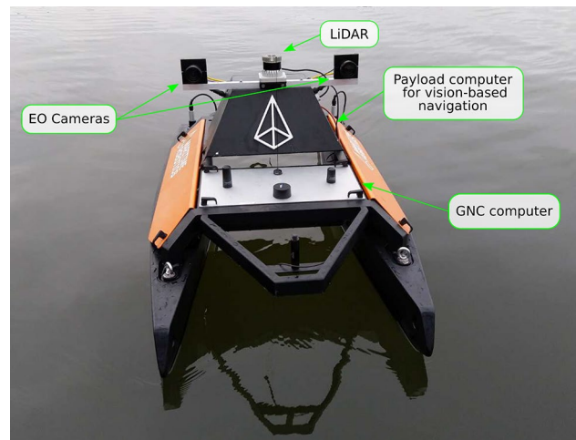
Fig. 1 The Otter USV from Maritime Robotics is armed with two (EO) cameras and a LiDAR for vision-based navigation. The guidance, navigation, and control (GNC) computer to control the vehicle is located in the grey box. The image is reproduced with kind permission of Maritime Robotics, https://www.maritimerobotics.com
