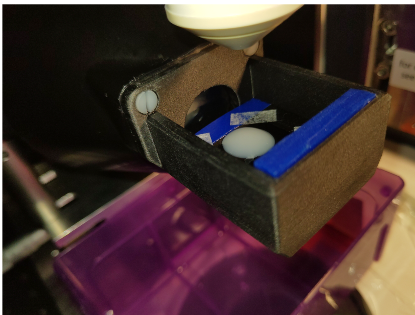
(b) Close-up of the sample holder, with a gel sample on a glass cover-slip installed. The sample is fastened with water-resisting tape to prevent it from moving around during measurements. The sample holder can easily be removed by loosening three white screws, and a plastic film separates it from the transducer cone which is filled with degassed water. As can be seen, half the ultrasound beam is blocked off, and acoustically absorbing material (blue) is used to prevent standing-waves. When measuring, the setup will be raised to submerge the objective, and filled with water.
