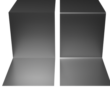
Figure 5.4: Two models with different edge geometry to showcase the effect different effects it has on shading and light reflections. Model on the left features sharp 90-degree edges, and the model on the right features smooth rounded edges.
