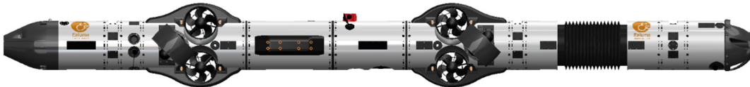
Figure 6.1: Image of the EELY500 robot provided by Eelume[11]. Note that the modules attached to the robot in this image is for illustration purposes and is not a 1:1 representation of NTNU's EELY500 robot.
