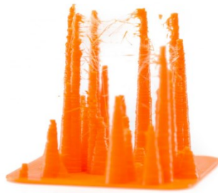
Figure 2.11: Illustration of stringing (Ultimaker, 2020e)
