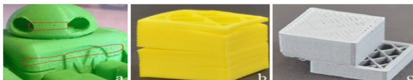
Figure 2.13: Layer defects (a) missed layers (b) separated layers (c) misaligned layers (Baş, Eevli and Yapıcı, 2019)
