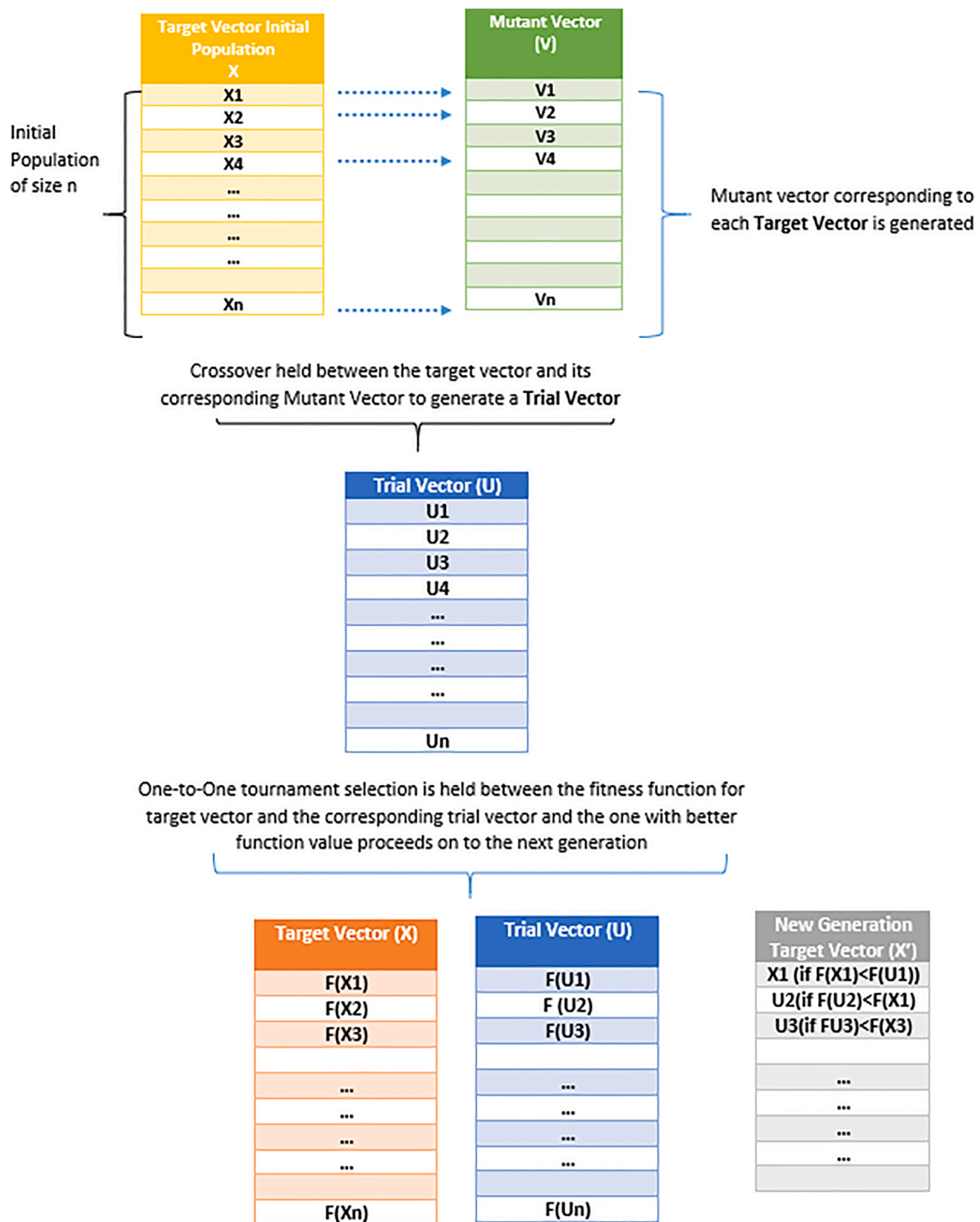
Fig. D.1. Diagram describing the details of the DE method used in this work.
