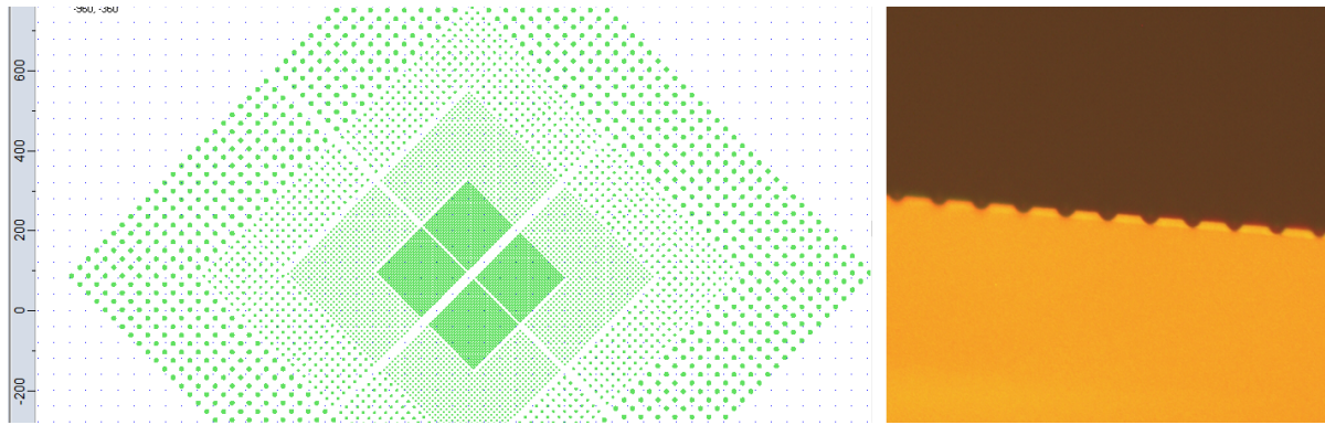
Fig. 3 Design of the mask (first image) for imaging the cross-section of the photoresist (second image). The features are circular with a diameter of 2 microns and the spacing between them decreases towards the central point to optimize the resolution. The coverslip is cut along the diagonal of the mask to reveal a cross-section of the microholes, magnification 50x.
