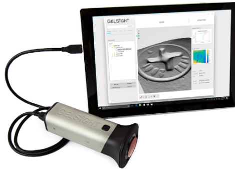
Figure 3.1: The GelSight Mobile acquired by Olympiatoppen. It consists of the GelSight instrument connected to a tablet/PC (GelSight, 2019)
