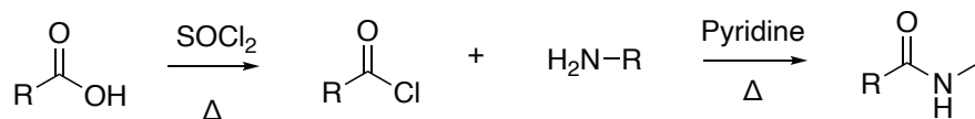
Scheme 1.13. Formation of an amide bond from a carboxylic acid and amine via acid chloride.
