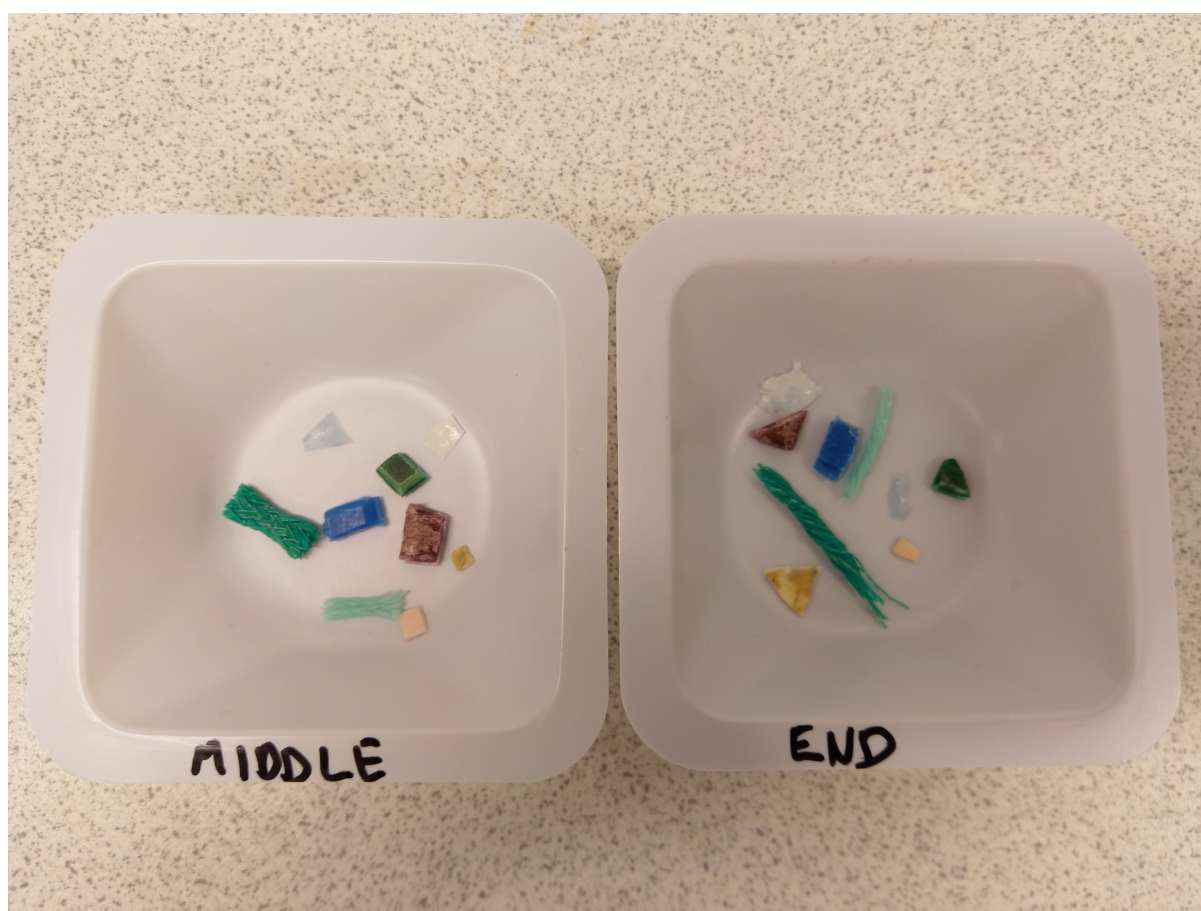
Figure 3.6: Samples from Isfjord Radio cleaned and cut for SEM analysis (before gold coating).
