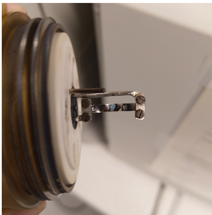
Figure 3.4: Plastic sample placed on the platinum filament.
