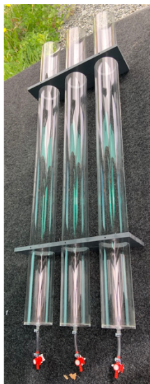
Figure 2.4 The three plexiglass pipes used for experiments.
