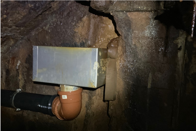
Figure A.8 The sampling point “second collection” where water is collected into pipes and being led directly to the threshold. Samples were taken of the water running along the wall and into the box.
