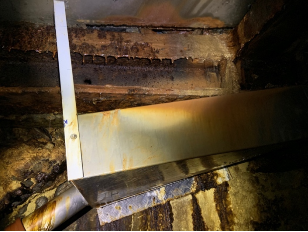
Figure A.7 The sampling point “first collection” where water is collected into pipes and being led directly to the threshold. Samples were taken of a thin stream of water, not visible in this picture, running into the box.
