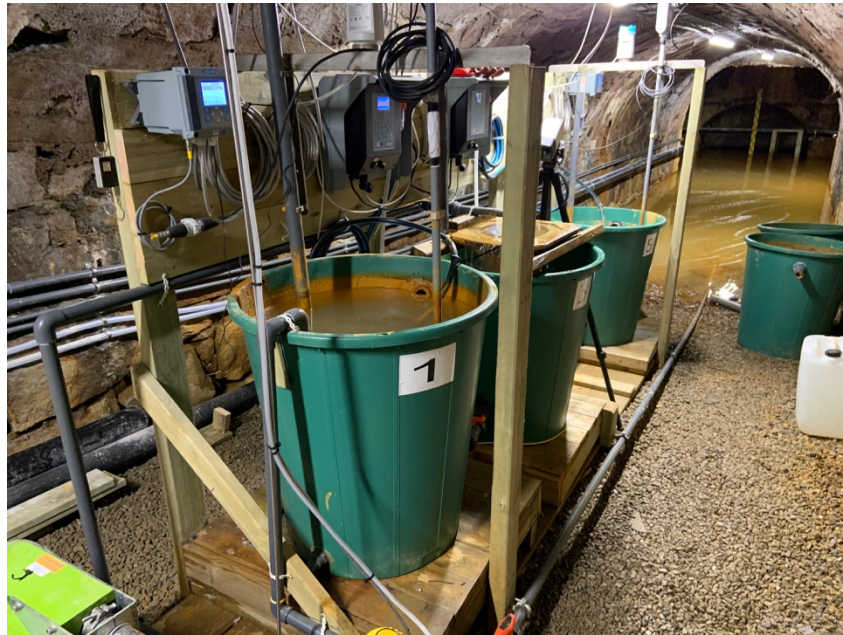
Figure A.2 The system after 29 th of January where the treatment medium, in this case olivine, was placed in an upside-down traffic cone in the middle tub.
