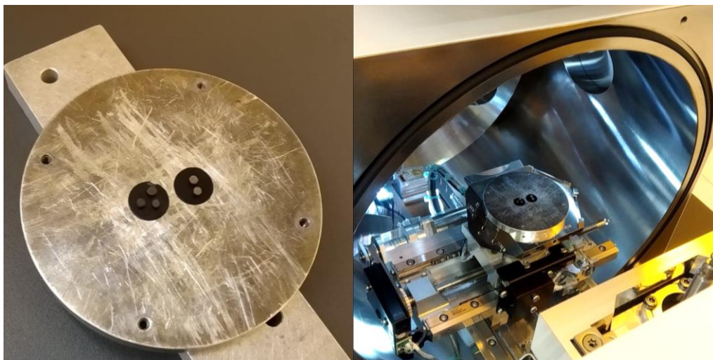
Figure 3.13 Cross-section pellets in stage holder (left) and loading to SEM Apreo (right).
