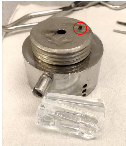
Figure 3.12 Iron holder and mounting wax. Pellet of about 1mm diameter rounded in red.
