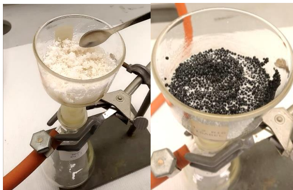
Figure 3.2 First impregnation (left) and second impregnation (right) of \gamma -Al 2 O 3 in a Büchner funnel with continuous manual stirring.
