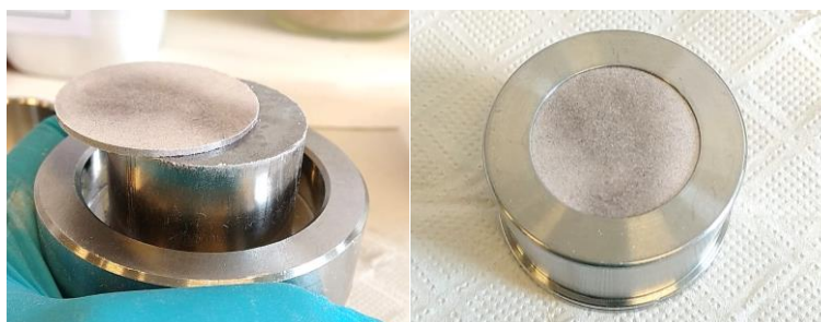
Figure 3.7 XRF pellet taken out from the iron pellet-form (left) and sample holder (right).
