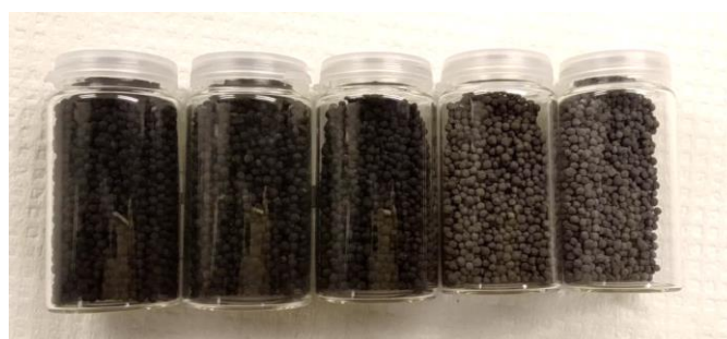
Figure 3.4 Target sorbents from EG-SQ method increasing Mo concentration from left (15Mn) to right (15Mn10Mo).
