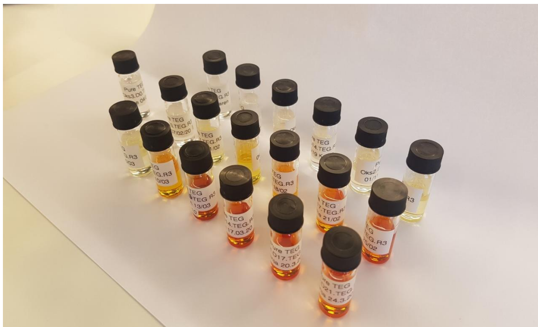
Figure 14 : We can see on this image the evolution of the colour of degraded TEG samples (R3). The background row corresponds to Oks 2 (100°C), the middle row to Oks 3 (120°C) and the front row to Oks 4 (140°C).
