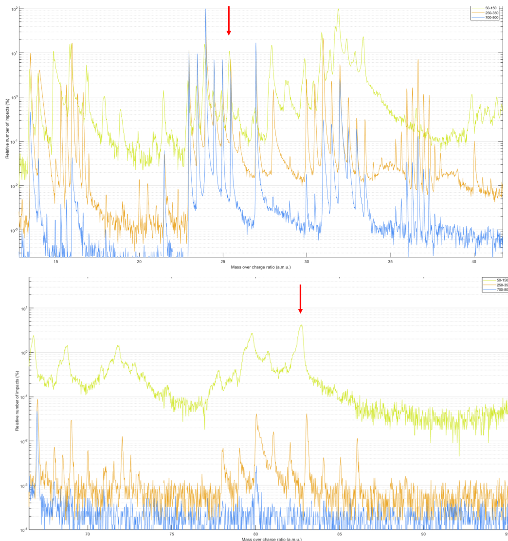
Figure 5.1: ROI mass spectra displaying the peaks at 25,5 and 83 respectively, marked with a red arrow. The green plot indicates the mass spectra in the region between 50-150nm, the orange plot annotates the mass spectra in the region between 250-350nm and the blue plot annotates the mass spectra in the 700-800nm region. The relative numbers of impact at the y-axis is in a logarithmic scale.
