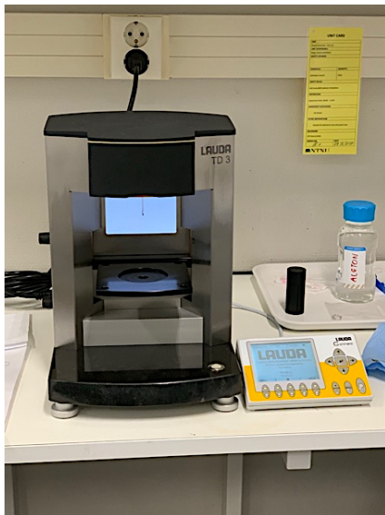
Figur 23: Platinum ringtensiometer (LAUDA TD 3)
