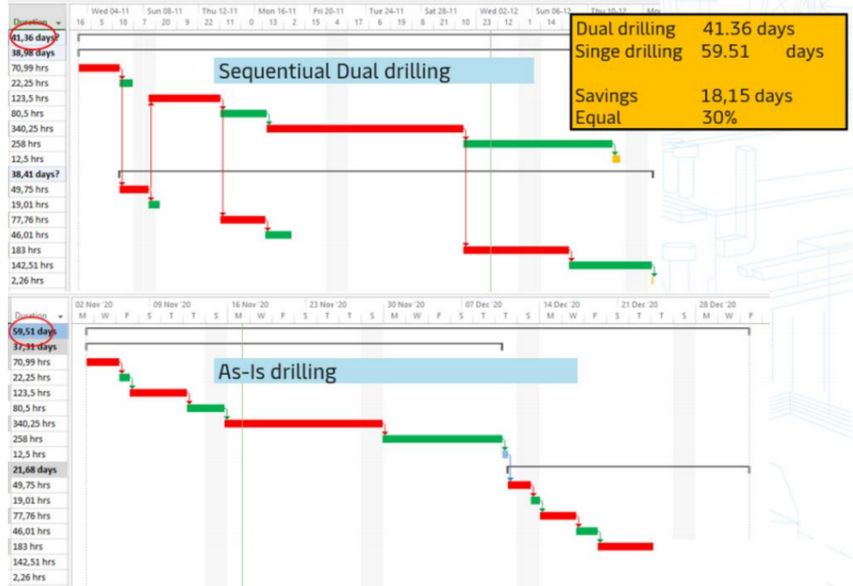
Figure 4: Time savings between dual drilling and conventional drilling from Jack ups.
