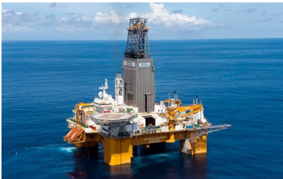
Figure 4: Semi-submersible rig Deepsea Stavanger w/ GVA 7500 design (Petroleumstilsynet 2017)
