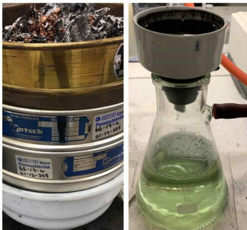
Figure 3.1 - Picture on left, sieving set-up and picture on right shows the vacuum filtration set-up.
