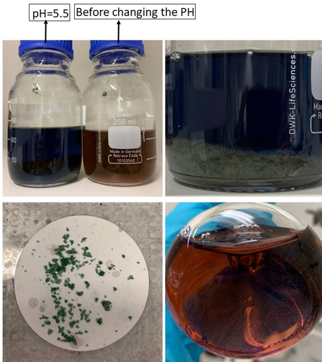
Figure 4.9 - Top left picture shows the change in the color of leachate after adjusting the pH to 5.5 by ammonia, the dark blue is the leachate at pH=5.5. Top right demonstrates the precipitates in the leachate. Bottom left shows the filter cake after filtration of 2 times diluted leachate. Bottom right shows the small precipitates in the leachates after multiple filtration.
