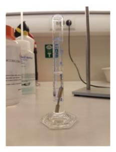
Figure 19: Setup for the density measurements using Archimedes' principle.
