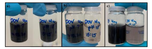
**Figure 5.7:** Colloid buffer solutions at pH 7 (left vial) and pH 10 (right vial) with pristine IFE Si NPs, (a) at the time of immersion, (b) after 1 day and (c) after 68 days. The present pristine NPs come from another production batch than used for other experiments, but they have similar morphology and size distribution. A concentration of 0.4 mg/mL was used for these test-vials.
