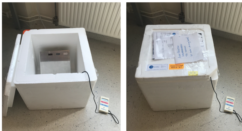
Figure 3.6: Pictures presenting the setup and the Styrofoam box used when comparing the de-icing properties of the 50/50 Cu/CuO and SiC prototype coatings.
