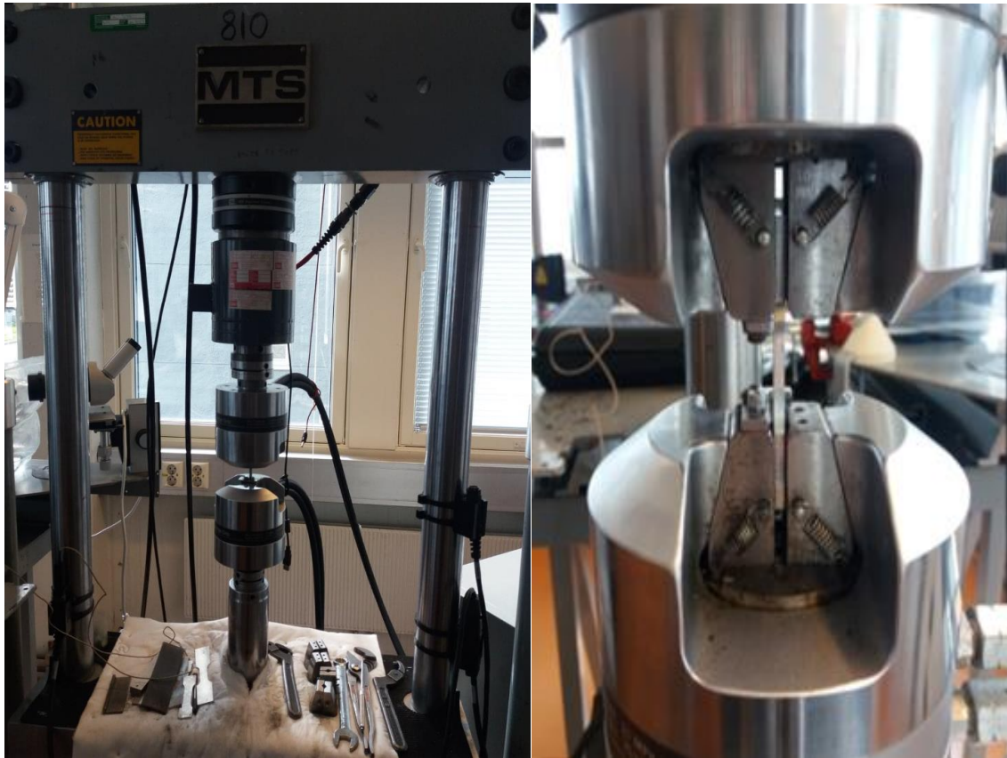
Figure 3.16: The setup of the fatigue test.
