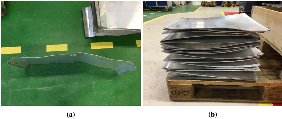
Figure 3.2: Extruded EN AW 6082.50 sheets (a) after four point bending in a hydraulic press, and (b) after the straightened sections were extracted.
