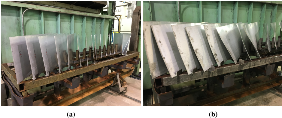
Figure 3.1: Extruded EN AW 6082.50 sheets (a) before solution heat treatment, and (b) after solution heat treatment and water quenching.
