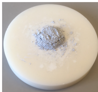
Figure 3.1: Sample encased in sacrificial powder on an alumina plate ready for sintering.
