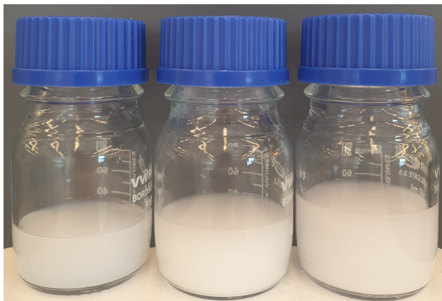
Figure 4.1: Image of the synthesized silica sols, with particle sizes of (from left to right) 95 \pm 11 nm, 192 \pm 24 nm and 256 \pm 40 nm.
