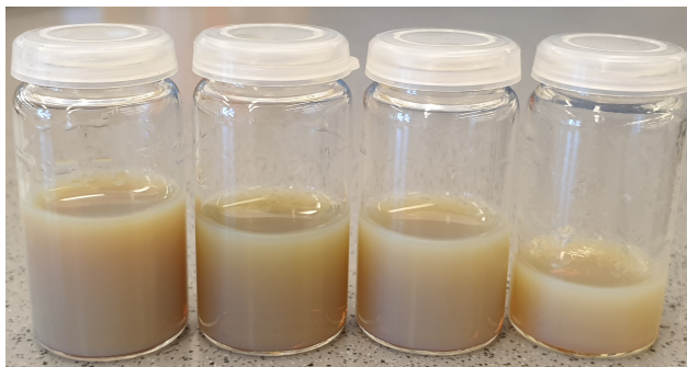
Figure 4.6: Image of the final colloids prepared by variations of the Lee-Meisel citrate method. From left to right, the AgNP#1, AgNP#2, AgNP#3 and AgNP#4 colloid.
