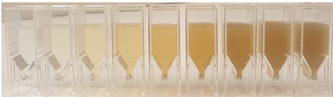
Figure 4.9: The color evolution of the AgNP#4 colloid prepared by the Lee-Meisel citrate method during the first 10 minutes of reaction. From left to right, a blank sample containing water and samples withdrawn at a boiling time of 3, 4, 5, 6, 7, 8, 9 and 10 minutes.
