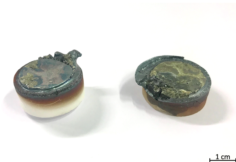
Figure 5.3: The samples after the second attempt at heat treating at 1300 °C for 3 hours. The slip-cast silica crucible is to the left and the quartz glass is to the right. The steel plate is melted and stuck onto both sample surfaces.
