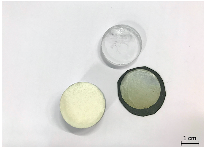
Figure 5.1: Samples C.900.24.1, Q.900.24.1 and the steel plate after heat treatment.
