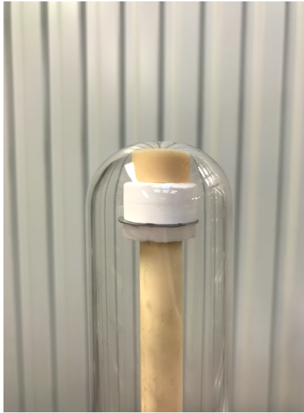
(a) Slip-cast crucible, steel and quartz glass samples placed in the quartz tube on top of the alsint pipe. An extra piece of the alsint pipe was added to the top of the diffusion couples to ensure intimate contact between the faces of the samples.
