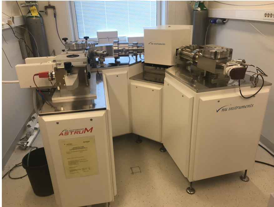
Figure 4.8: The Astrum GD-MS by Nu Instruments used to analyse the iron distribution in the heat treated samples.
