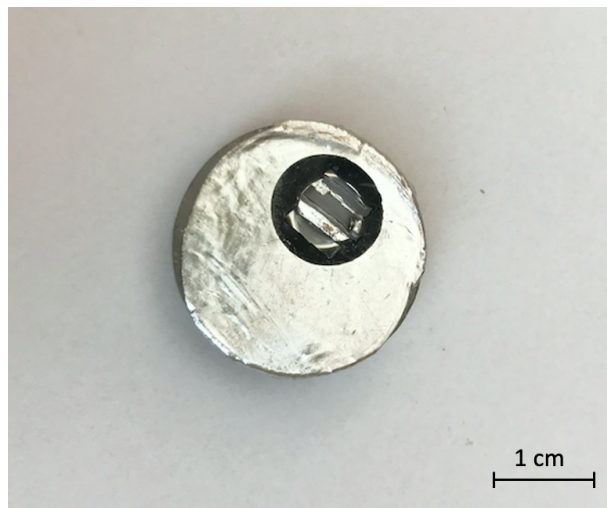
(a) A quartz glass sample with the indium mask after the GD-MS analysis.
