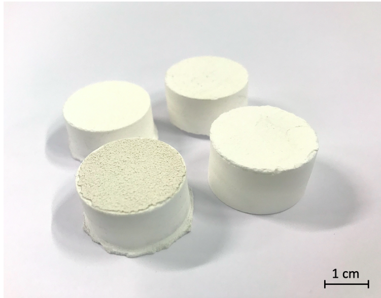
Figure 4.1: Samples of the Vesuvius slip-cast crucible. The sample in the front left is coated.
