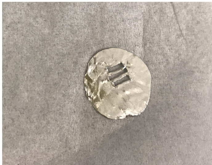
Figure 4.10: The 7N purity indium mask prepared for GD-MS analysis. Small areas are cut out so the sample can be sputtered.
