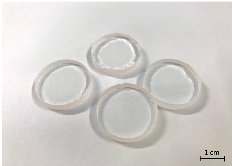
Figure 4.3: Quartz glass samples prepared by the glassblower workshop at NTNU.
