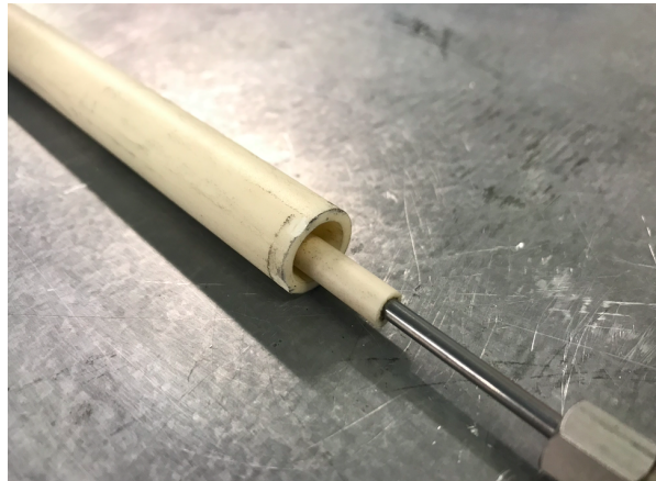
(b) An additional closed-end alsint pipe was added inside the original alsint pipe to protect the thermocouple from oxidising.
