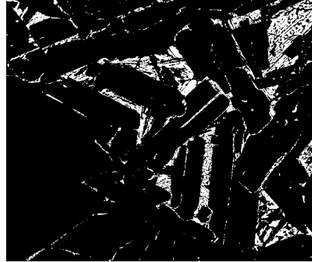
(b) Total area of only the white phase in the metal from sample 45-55-24-1. The image is taken at 40x.
