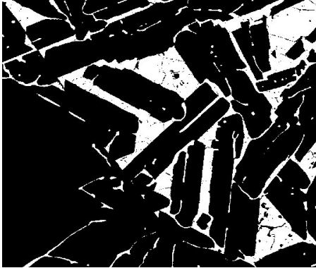
(a) Total area of the \text{Si}_2\text{Ca} and \text{Si}_2\text{Al}_2\text{Ca} phase in the metal from sample 45-55-24-1. The image is taken at 40x.
