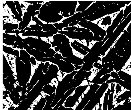
(b) Total area of only the Si 2 Al 2 Ca phase in the metal from sample 35-65-2. The image is taken at 40x.
