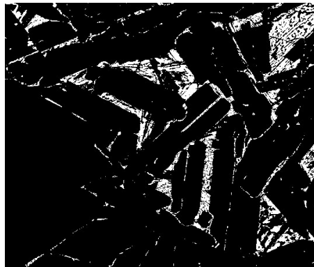
(b) Total area of the white phase in sample 45-55-24-1. Analyzed at 40x.
