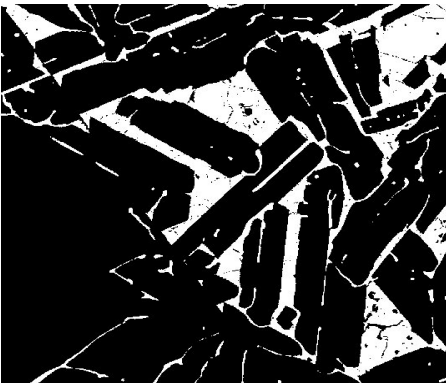
(a) Total area of the white and light-grey phase in sample 45-55-24-1. Analyzed at 40x.
