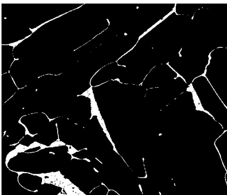
(a) Total area of the white and light-grey phase in sample 45-55-180-1. Analyzed at 40x.
