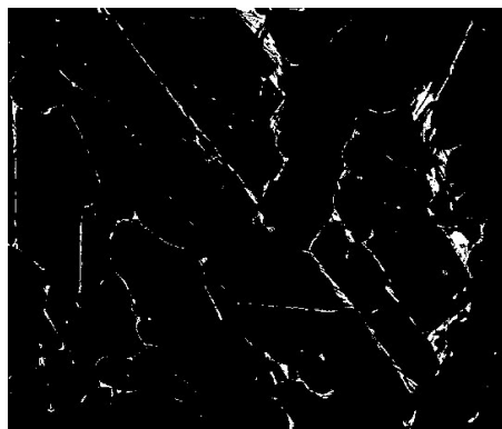
(b) Total area of the white phase in sample 45-55-60-1. Analyzed at 40x.
