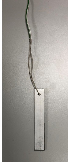
Figure 4.2: setup of thermocouple to measure cooling rates, the two threads in the thermocouple is welded together through a hole in the sample.
