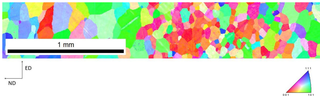
Figure 6.1: IPF map through the thickness from the author's project thesis. Scan is parallel to the TD axis.
