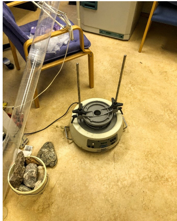
Figure 26 Mechanic shaker used in the sieving analysis
