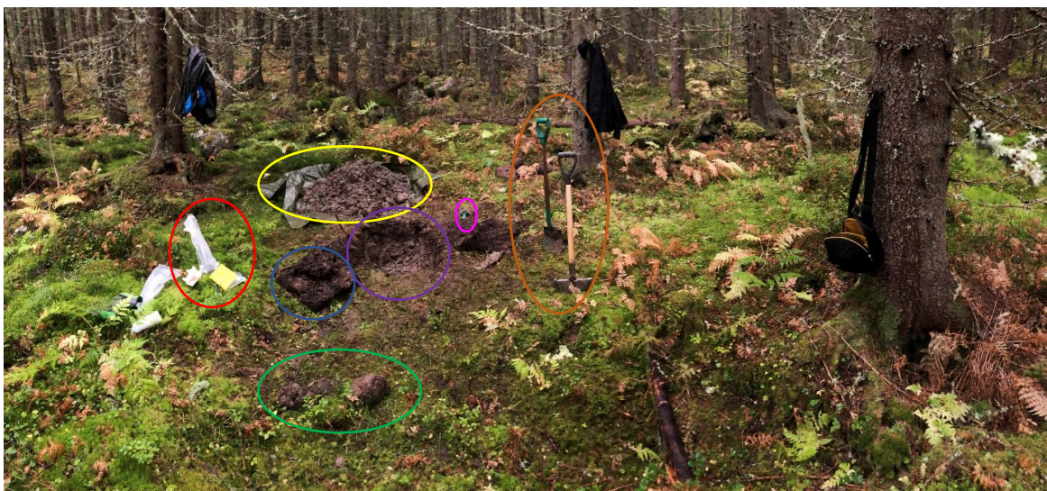
Figure 24 Overview of the sampling procedure in field. Green circle: bigger rocks manually sorted out. Blue circle: intact surface cover to cover up after digging. Red circle: plastic bags to store samples and field notebook. Purple circle: Sampling hole. Orange circle: shovels to dig the hole. Pink circle: Gardening shovel to collect the sample. Yellow circle: tarpaulin to collect sediments.
