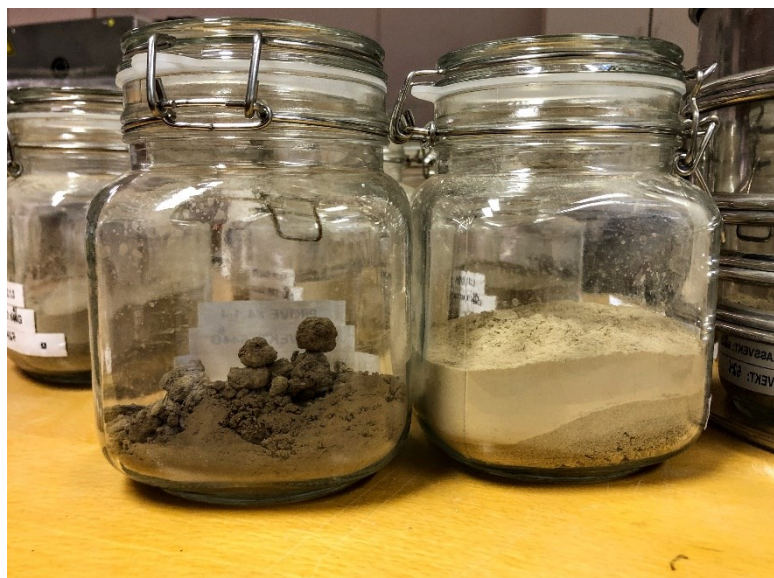
Figure 27 Samples before (to the left) and after (to the right) sieving
