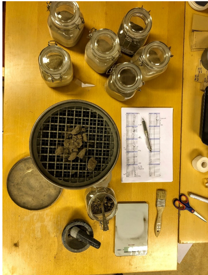
Figure 25 Stacked sieves, mallet, brush, weight, spoon, brush, spreadsheet and samples used in sieving analysis
