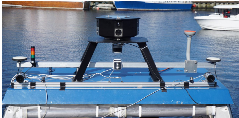
Figure 6.3: Sensors mounted on milliAmpere
