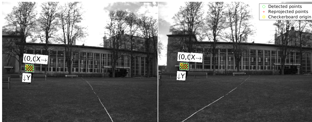
Figure 8.2: Corners of checkerboard detected
