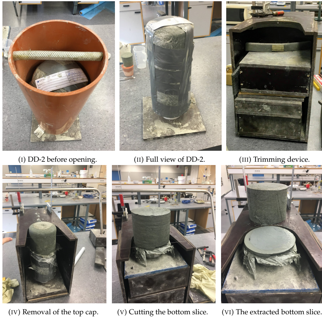
FIGURE 4.5: General opening and trimming procedure of a mini-block sample into cylindrical slices.
