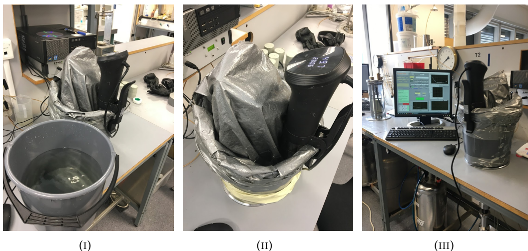
FIGURE 5.6: Heating sleeve operation. (I) Pouring water from another bucket into the tarpaulin. (II) Mounting the immersion circulator and starting it by selecting temperature and time settings on the touch pad. (III) Full view of the triaxial apparatus wrapped with the heating sleeve.
