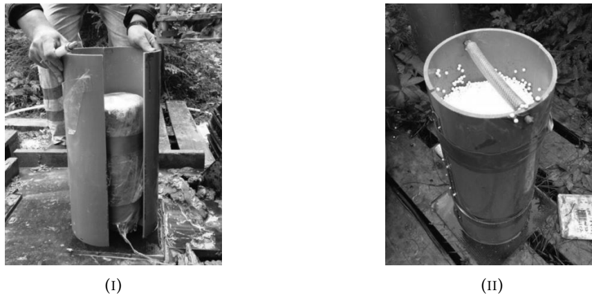
FIGURE 4.2: Sample protection and transportation. (I) PVC tubes for transport. (II) Transport tube containing sample and styrofoam balls. Modified from (Emdal et al., 2016).
