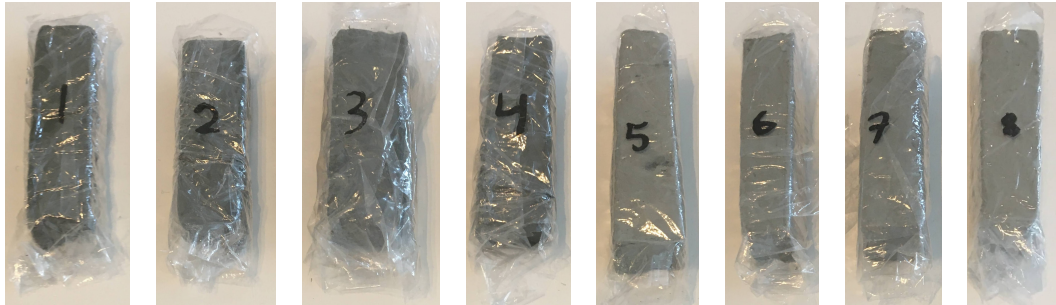
FIGURE 6.3: Photographs of the micro-CT specimen before the first scan. S1 - S4 were stored in a fridge, while S5 - S8 were heated to 70 \text{ }^\circ\text{C} before being stored at room temperature.
